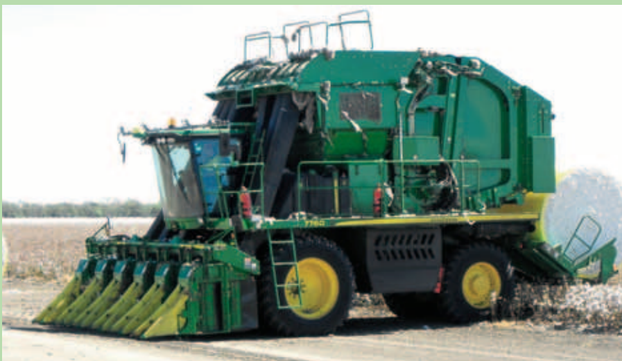
A mix of excitement and enthusiasm was evident as the John Deere 7760 Round Module Builder, the next generation cotton picker, combining harvesting and module building solutions into one versatile cotton harvester, was put through it's paces at Bullaman Plains, Thallon.
